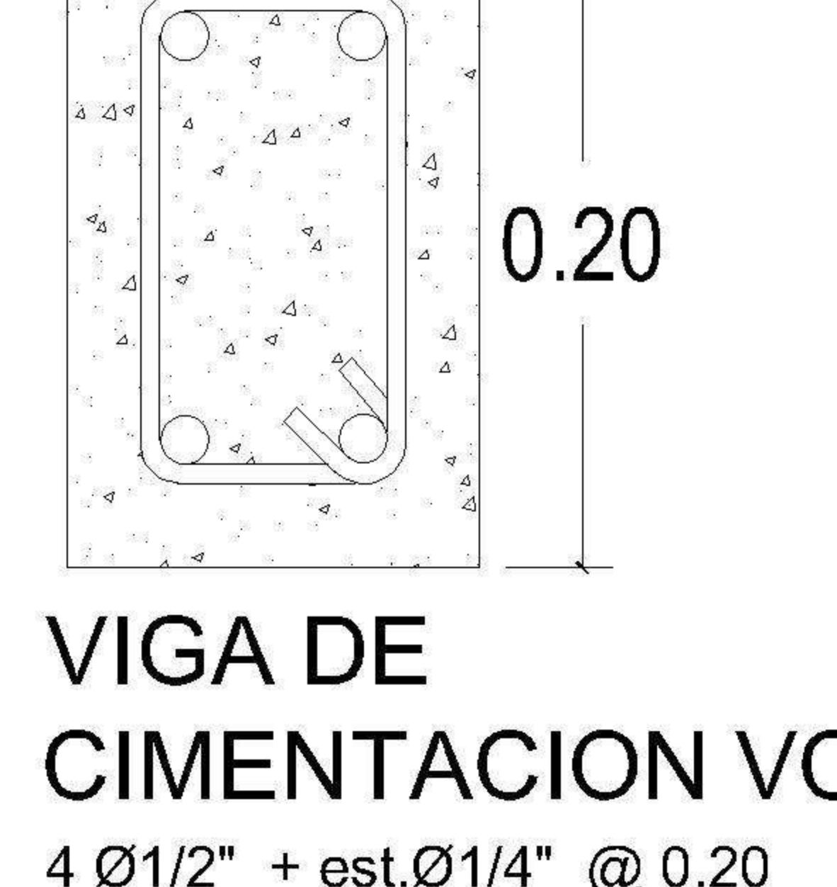
VIGA DE CIMENTACION VC 4 Ø1/2" + est. Ø1/4" @ 0.20
